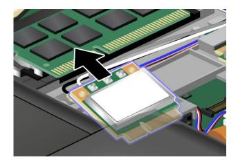
8. Align the contact edge of the new PCI Express Mini Card with the corresponding socket contact of the computer.
